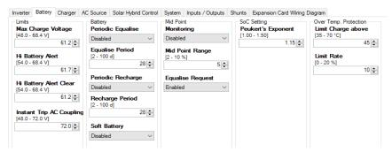
Max Voltage Limit is the absolute maximum voltage produced by the charging section of the inverter in any charge stage.
