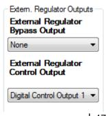
The AC Coupled Inverter Output drives an external solid state relay to control when the AC Coupled inverter feeds to the grid, local AC Load and battery bank. This is suitable for switching any Grid feed inverter. This setting is only available for Solar Hybrid (grid connected) configurations.
