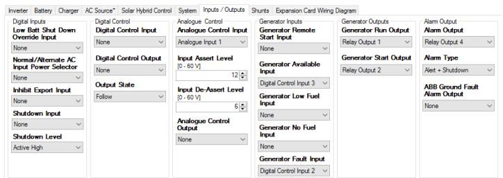
Low Batt Shutdown Override Input function is also known as the "Just Go" control. In case of emergency, even if the batteries would normally be considered too flat to safely run the inverter, activating this input will force the inverter to run, until there is insufficient battery power left to maintain the load. This is considered essential if, say, phones or a fire pump MUST be operated.
