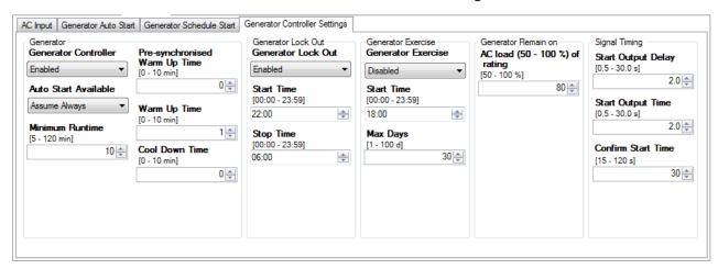
If there is an automatic generator permanently connected to the system the **Generator Controlle**r setting should be set to Enabled. This is highly recommended for OFF Grid systems. If there is no automatic generator connected it should be Disabled
