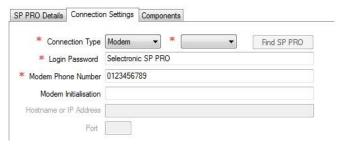
For Modem connections, select the PC COM port that the modem is connected to. Enter the MODEM PHONE NUMBER. This is the number that SP LINK will dial when you select Connect. Modem Initialisation can be left blank when using Selectronic supplied modems but may be required for other modem types. Consult the modem supplier if unsure.
