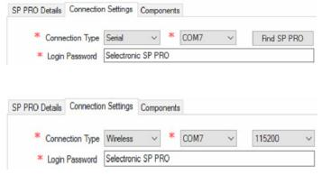
Use DIRECT connection Type when using a RS232 serial connection. Once all cables are connected and in place, press FIND SP PRO - this will search through all PC ports and find the connected SP PRO and set connection parameters.
