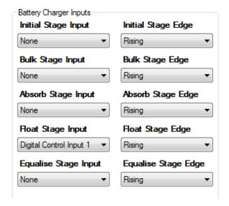
Float Stage Edge Consult the regulator manufacturer to determine the output signal the chosen regulator provides. The most common is the default of Rising edge.
