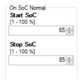
The ON SoC NIGHT ASSIST state of charge control monitors the State of Charge through the highest usage period, usually during the evening. If the battery level has dropped to the **Start SoC** level at the appointed time (between the Start Time and the Stop Time)the SP PRO will start the generator and raise the state of charge until the batteries reach the Stop SoC level. This prepares the system for the night ahead.
