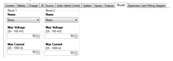
The Shunts tab contains settings required to configure the connected DC current shunts that are used to measure the currents going in or out of the battery bank. The shunt readings are used by the SP PRO series to accurately calculate the state of charge of the batteries (System SoC).
