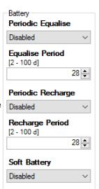
**Soft Battery** setting is used with battery banks that are "soft" meaning they have a relatively high internal impedance. Useful with aqueous type battery technologies or battery banks with high internal impedance. Technically this function is achieved within the SP PRO by reducing the gain of the battery charger's voltage control loop thereby increasing the damping of said loop. Soft setting reduces the gain to 50% whilst Very Soft to 25% of the normal value.
